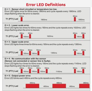
Error LED blinks periodically when an error condition occurs. The charts above are created as sample for T1(PT1) LED indicator. Similar denotions are valid for T2 (PT2), T3 (PT3) and T4 (PT4) LED indicators.
