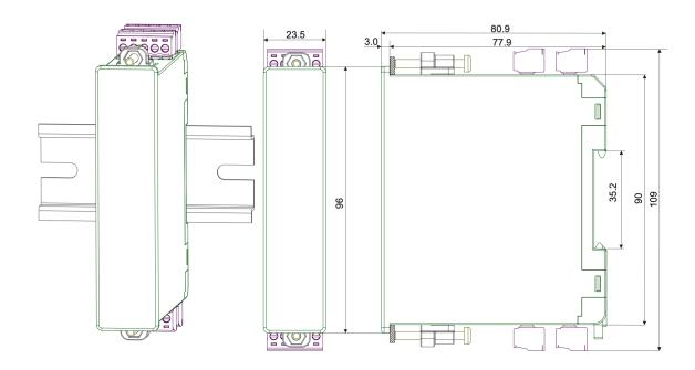
NOTE: The unit of measurement is millimeters.
