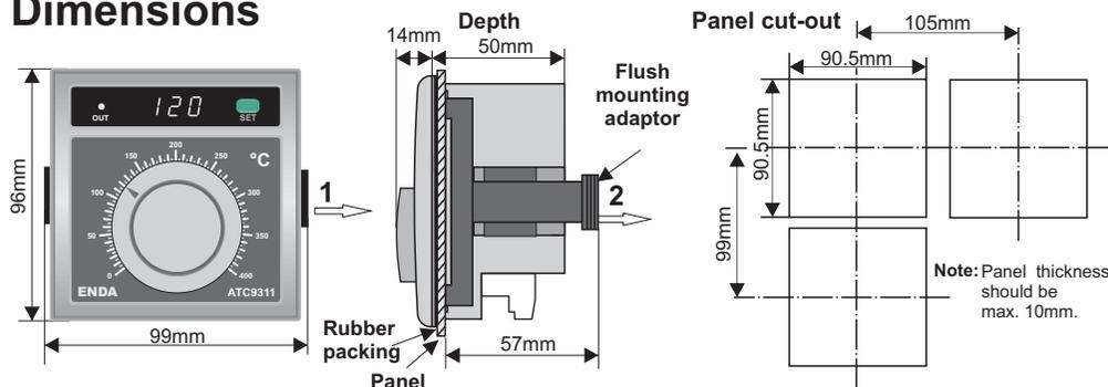
**For removing mounting clamps :** Push out the flush-mounting clamp in direction 1 as shown in the figure above. Then, pull out the clamp in direction 2. If there is no 60mm free space at back side of the device, it would be difficult to remove it from the panel.
