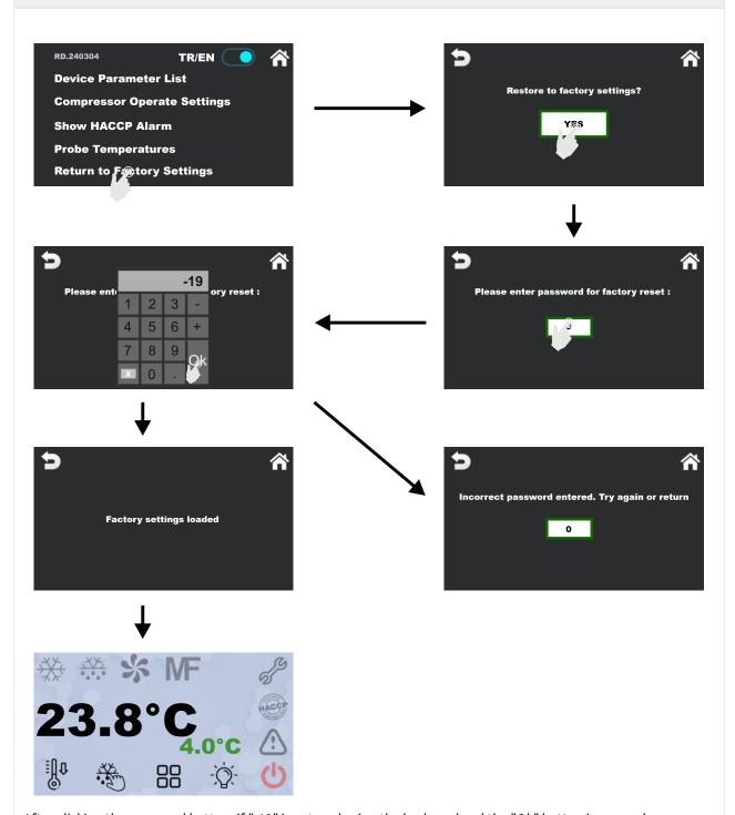
After clicking the password button, if "-19" is entered using the keyboard and the "Ok" button is pressed, a message indicating that the password has been entered correctly will be displayed on the screen for 2 seconds. Then, the device will return to the "Main Screen" and start operating according to the factory settings. If the password is entered incorrectly, a "Incorrect Password Entered" warning will appear, and the password will need to be entered again.
