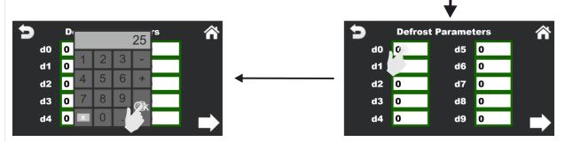
To enter the "Parameter Menu", you need to click on the Device Parameter List. While in the "Parameter Menu", clicking on the text corresponding to the parameter opens the relevant parameter page. If you click on the text "Defrost", it enters the defrost parameter menu.
