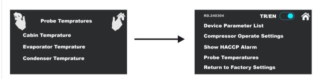
While in the configuration screen, clicking on the text Probe Temperature Display enters the screen where probe temperatures are displayed.
