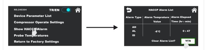
While on the configuration page, clicking on the Show HACCP Alarm text navigates to the page where HACCP alarms are displayed. Here, the temperature values at which the alarms occurred and the duration for which they remained active can be viewed. If the vest button is clicked, all generated alarms will be deleted.
