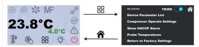
When the device is on the main screen, clicking the  $\begin{array}{c} \Box \\ \Box \\ \end{array}$  button enters the configuration screen.
