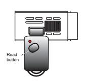
While in "Running Mode", if vevo n device or "Read" button on "ENDAKEY" is pressed, "dL" message appears on display and parameters are read and transferred to the device. If the parameter transfer is successful, the " r EF " message appears and the device begins to work with the loaded parameter values. If the parameters are wrong, incorrect or " ENDAKEY " is faulty,  $\mathcal{Err}$  " message appears. Parameters will not be changed on device.
