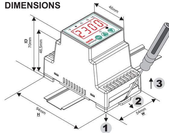
**Mounting the device to the rail :**
