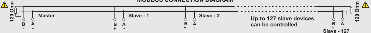
Termination should be accomplished by attaching 120 Ohm resistors to the start and at the end of the communication line.
