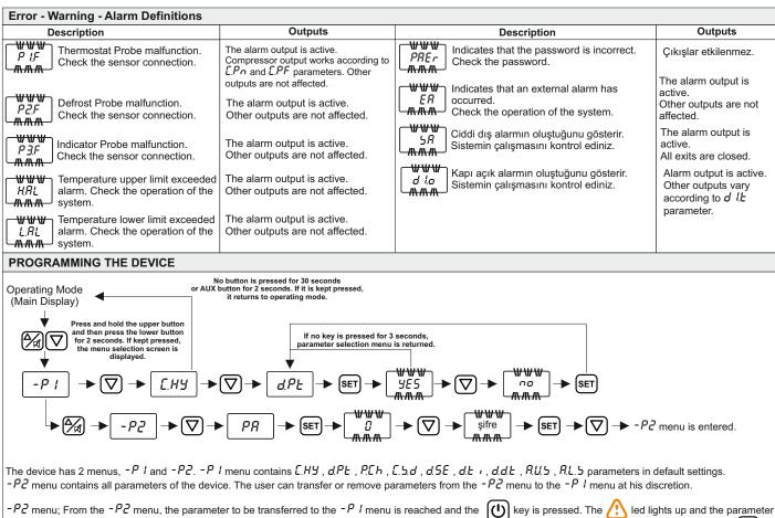
is transferred to the -P / menu. To remove the transferred parameter from the -P / menu, navigate to the relevant parameter in the -P2 menu and press the 😃 - P2 Password: "- 19 " key. The 🚺 led turns off and the parameter is removed from the -P *l* menu.
