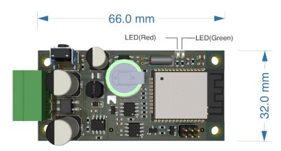
**Motage:** 1: Mount using M3 screws.
