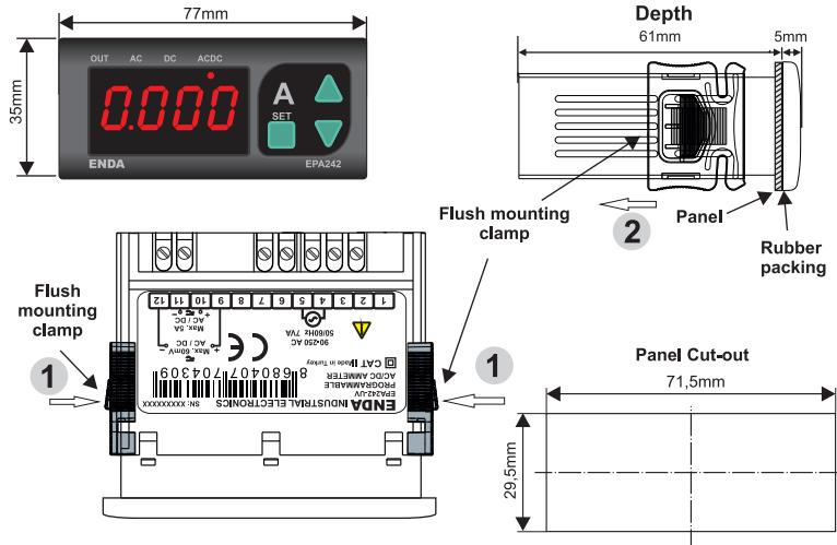
To removing mounting clamps :
