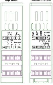
The logic output of the instrument is not electrically insulated from the internal circuits. Therefore, when using a grounded thermocouple, do not connect the logic output terminals to the earth.
