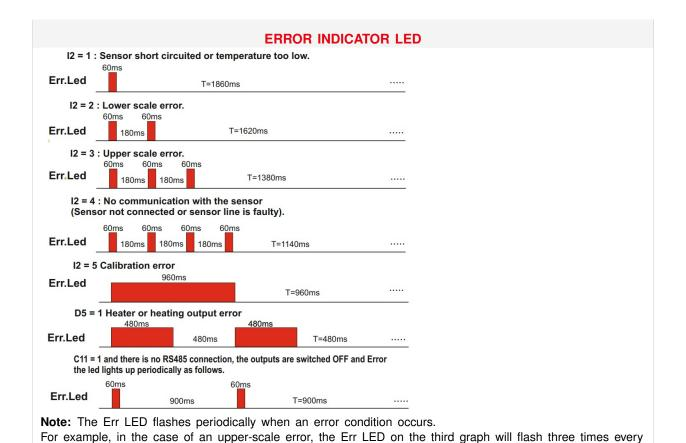
180 ms for a duration of 60 ms, and this cycle repeats after 1380 ms. When the error is resolved, the LED
