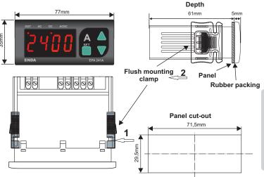
For removing mounting clamps:
