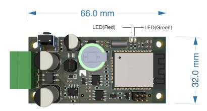
**Motage:** 1: Mount using M3 screws.
